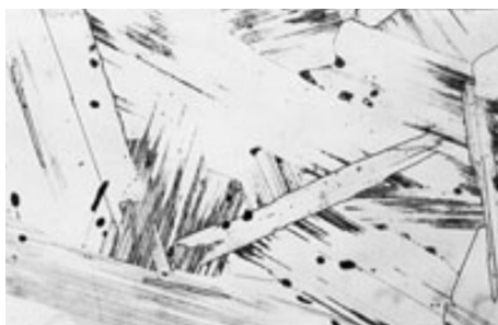
Fig. 2 \text{Os}_{40}\text{B}_{60} , arc melted and annealed at 1550^\circ\text{C} , 10 h; \text{Os}_2\text{B}_3 (dark)+ \text{OsB}_2 (light), etched; \times 500
